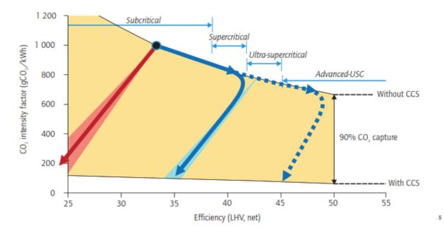
Since the late 1990s, there have been coordinated research efforts in many countries to push thermal cycle efficiencies even higher than ultra-supercritical into the so-called advanced ultra-supercritical range. However, since even the high-performance steels used in the
