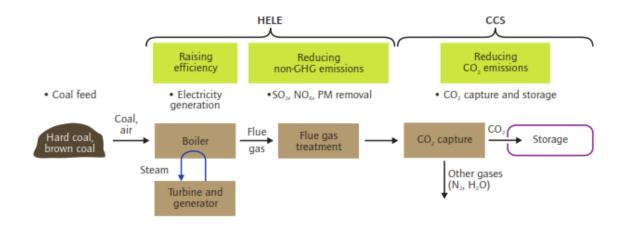
I first discuss pulverized coal combustion technologies, with varying efficiencies of the thermal cycle, followed by some of the other HELE technologies noted in the 2019 IRP. I conclude that ultra-supercritical efficiency is the highest possible cycle efficiency that can be anticipated for procurement of 1500 MW of new coal under the 2019 IRP and the Ministerial determination for 1500 MW of new coal.
