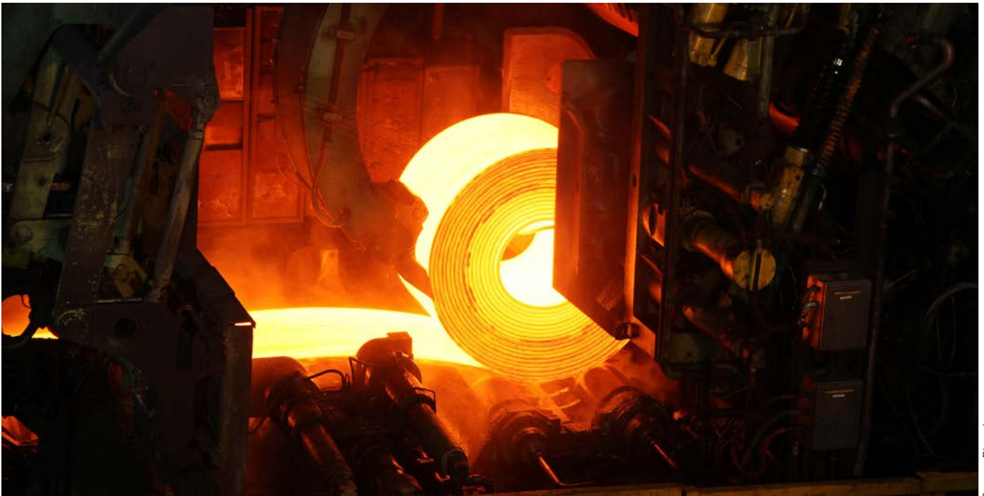
Red-hot rolled steel coil being run through rollers
