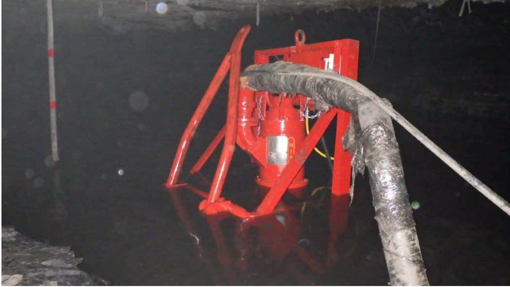
The skid mounted HIPPO Flameproof Submersible Slurry Pump System® in underground operation in a typical coal mine
