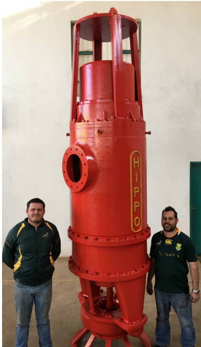
The HIPPO High Volume; High Head; Medium/High Voltage Flameproof Submersible Slurry Pump®
