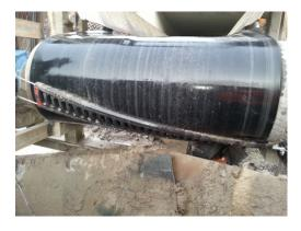
CleanScrape forms a three-dimensional curve beneath the discharge area that conforms to the pulley's shape.
