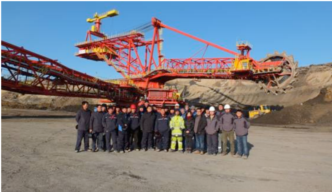
Fig. 1 (People.jpg): 6,600 m 3 /h Tenova TAKRAF Bucket Wheel Excavator at Zhahanaoer Open Pit Mine in China.
