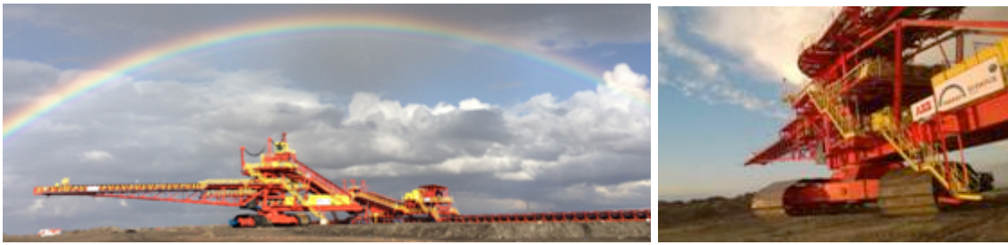
Fig. 2 & 3 (Rainbow.jpg, Spreader.jpg): 7,900 m 3 /h Tenova TAKRAF Spreader at Zhahanaoer Open Pit Mine in China.
