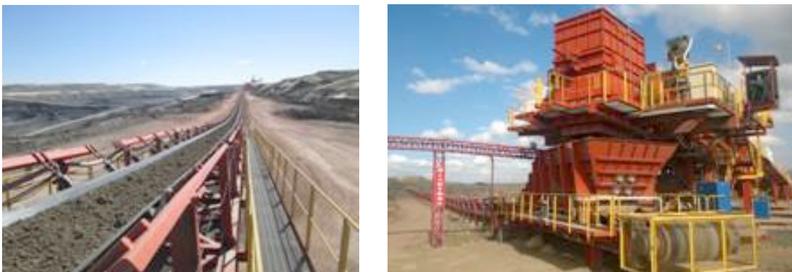
Fig. 4 & 5 (Conveyor1.jpg, Conveyor2.jpg): 7,900 m 3 /h Tenova TAKRAF Conveyor system at Zhahanaoer Open Pit Mine in China.
