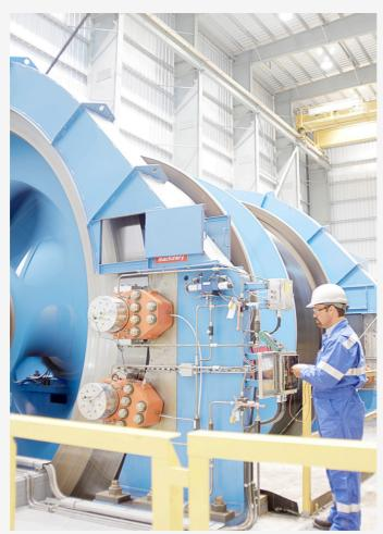
Hoist Performance Fingerprint — expert hoist condition check
