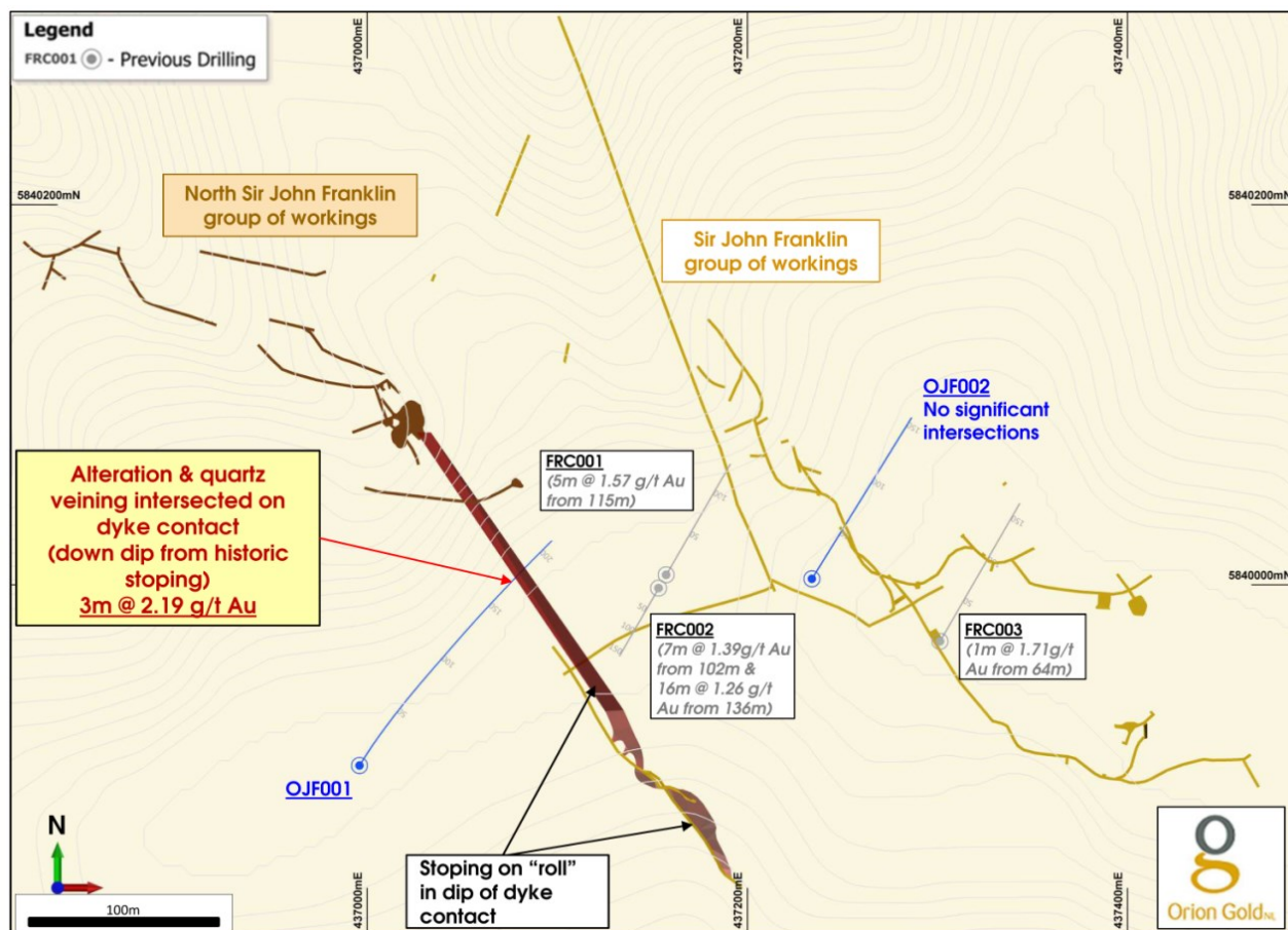
Figure 6: Sir John Franklin underground historical workings and reverse circulation holes completed in 2013 as well as historical drill results.
