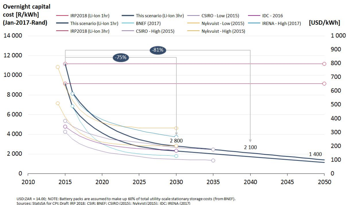
Figure 24: Overnight capital cost of stationary storage (excludes pumped storage) considered for the stationary storage scenario
