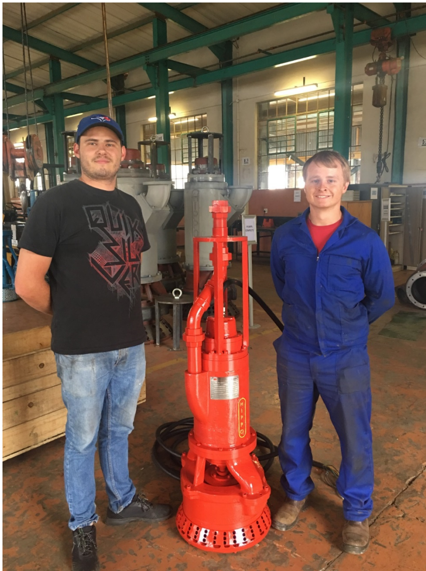
Marius Sunkel and Wayne Kelly flanking the 75L SBO HIPPO Bottom Suction Flameproof Submersible Slurry Pump ready for export to Houston
