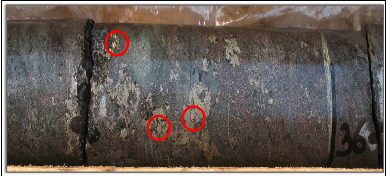
Close-up of IPC0003 disseminated sulphide zone at 36.00m down hole. Sulphides are a mix of pyrite and pyrrhotite with trace chalcopyrite (red circles).
