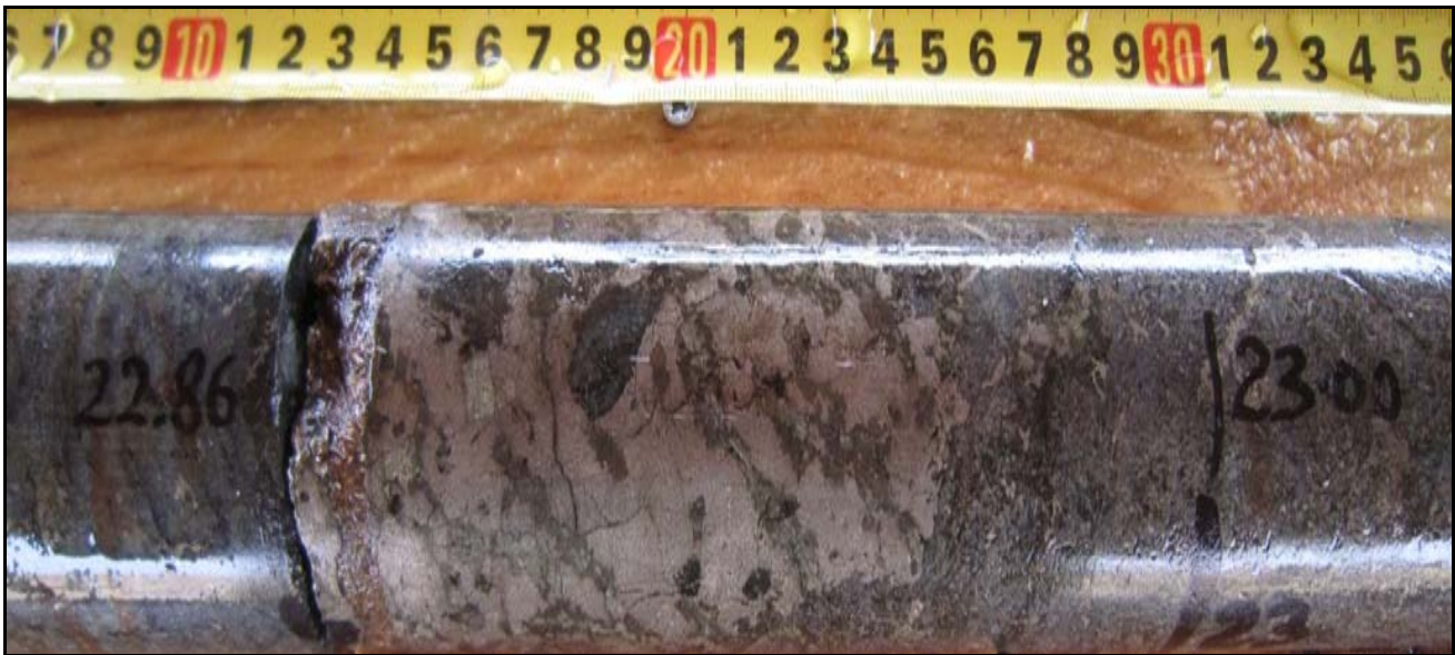
Close-up of IPC0004 massive sulphide band at 23.00m down hole – located within a 10m zone of (2-10%) disseminated sulphides. Sulphides are primarily pyrrhotite with lesser pyrite, with trace chalcopyrite observed elsewhere in the zone.
